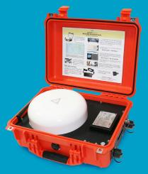
The MCD-4800 is an auto-pointing BGAN satellite terminal in a closed hardened case
