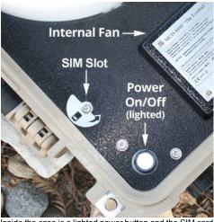
Inside the case is a lighted power button and the SIM card tray. The internal fan helps keep electronics cool if tempretures rise. It is recommended to open the case to help vent excess heat buildup in hot weather.
