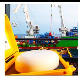
Inside the case is the auto-pointing antenna which is excellent for ocean going vessels and oil rigs. With the lid open or closed, the terminal operates for up to 5 hours on internal battery, or continuously if power is available.
